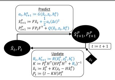
Figure 13: The Neural Kalman Filter (NKF). Differences from Fig. 1 are highlighted.  $\Delta t$  is constant; G, Q are the outputs of an LSTM network with hidden state  $h_a$ ; and R is the output of an LSTM with hidden state  $h_r$ .
