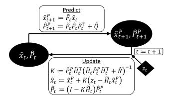
Figure 1: The KF algorithm. The prediction step is based on the motion model  $\tilde{F}_t$  with noise  $\hat{Q}$ , whereas the update step is based on the observation model  $\tilde{H}_t$  with noise  $\hat{R}$ .
