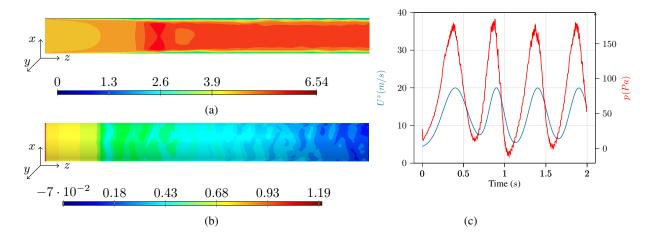
Figure 1. (1a): The velocity field profile  $\|\mathbf{U}\|_2$  of gas flow (m/s) in a pipeline. (1b): The pressure field of gas flow to the inner wall. (1c) The inlet velocity  $U^z$  and the mean inner wall pressure p of the whole pipeline through time. The periodic profile for  $U^z$  is suitable to imitate the real-life demand (Su et al., 2019).
